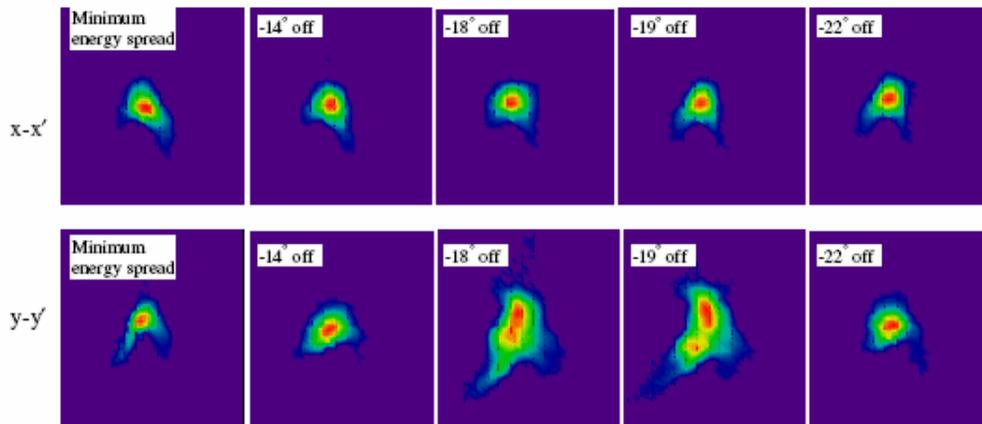
Reconstructed transverse phase space for varying beam parameters (optimal compression at -19 deg)
