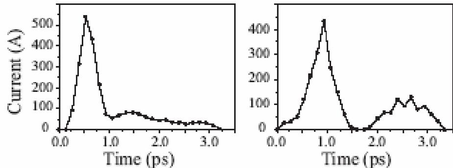
Longitudinal Distribution for compressed (left), and over-compressed (right) cases.
