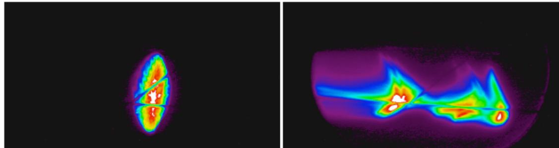
Min. energy spread and no compression - 9 deg fwd of crest (left); Max. compression -19 deg fwd of crest (right).
