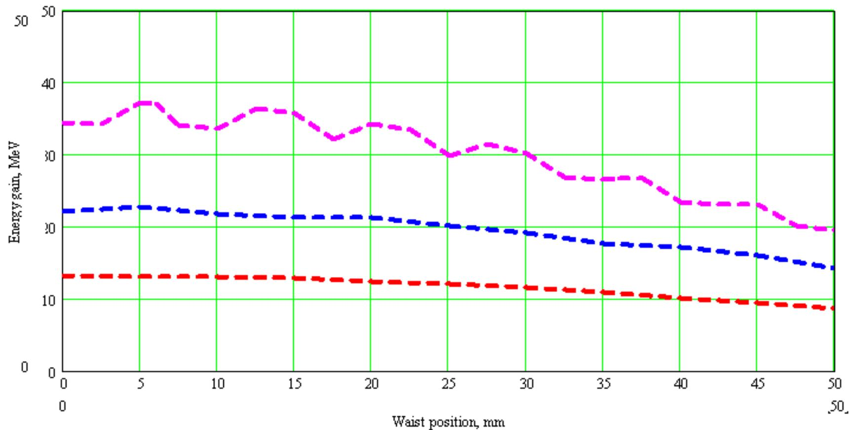
**FIG 3: Energy gain (MeV) vs. the waist position (mm)** when the magnetic field is always constant, and the laser power is 0.8 TW (note that “zero” corresponds to the magnet middle plain)
