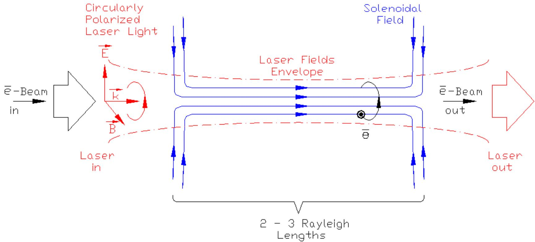
**FIG. 2:** Inside the solenoid
