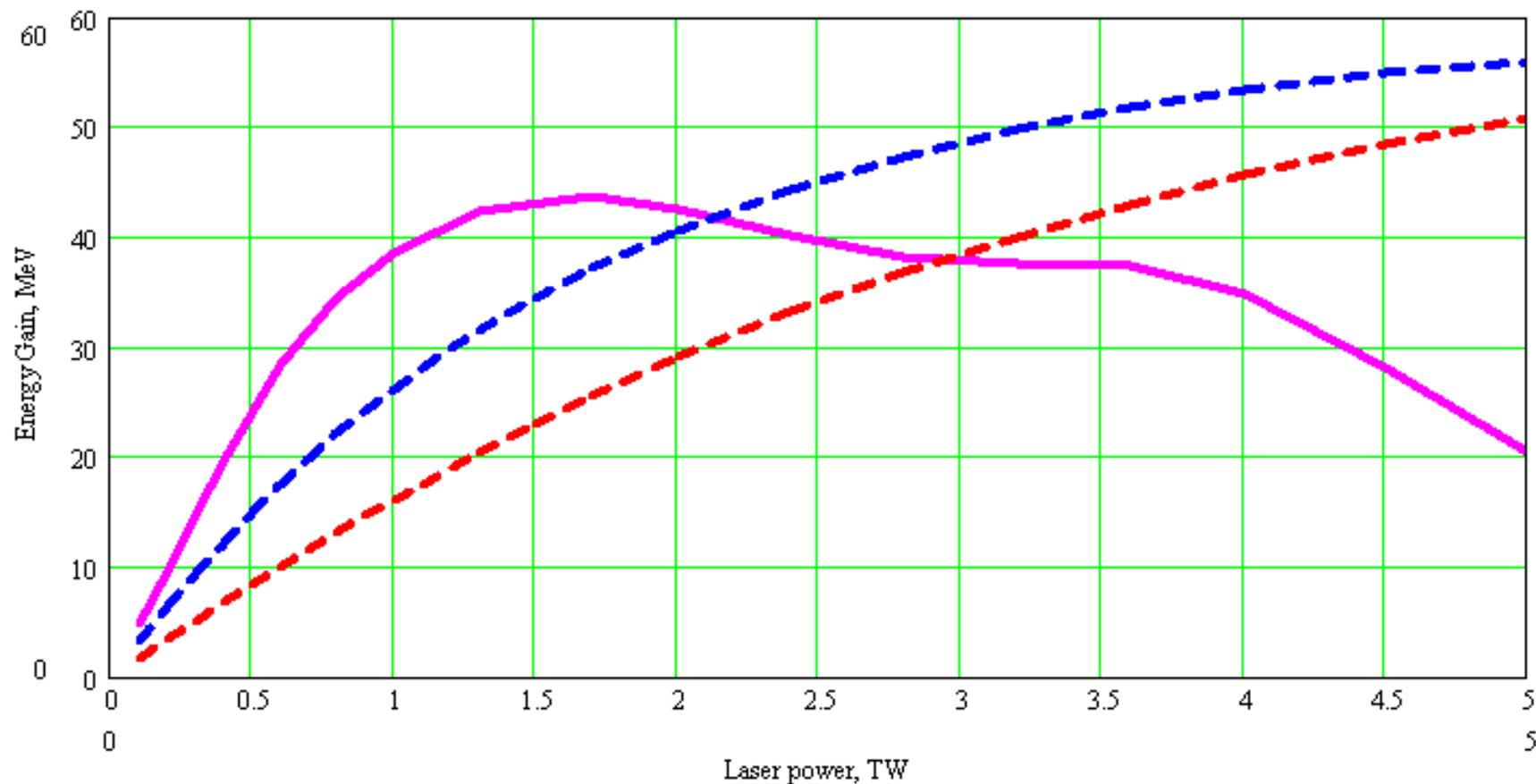
**FIG 2: Energy gain (MeV) vs. the laser power (TW)** when the magnetic field is always constant (the laser light is focused in the magnet middle plane with  $w = 1.3$  mm)
