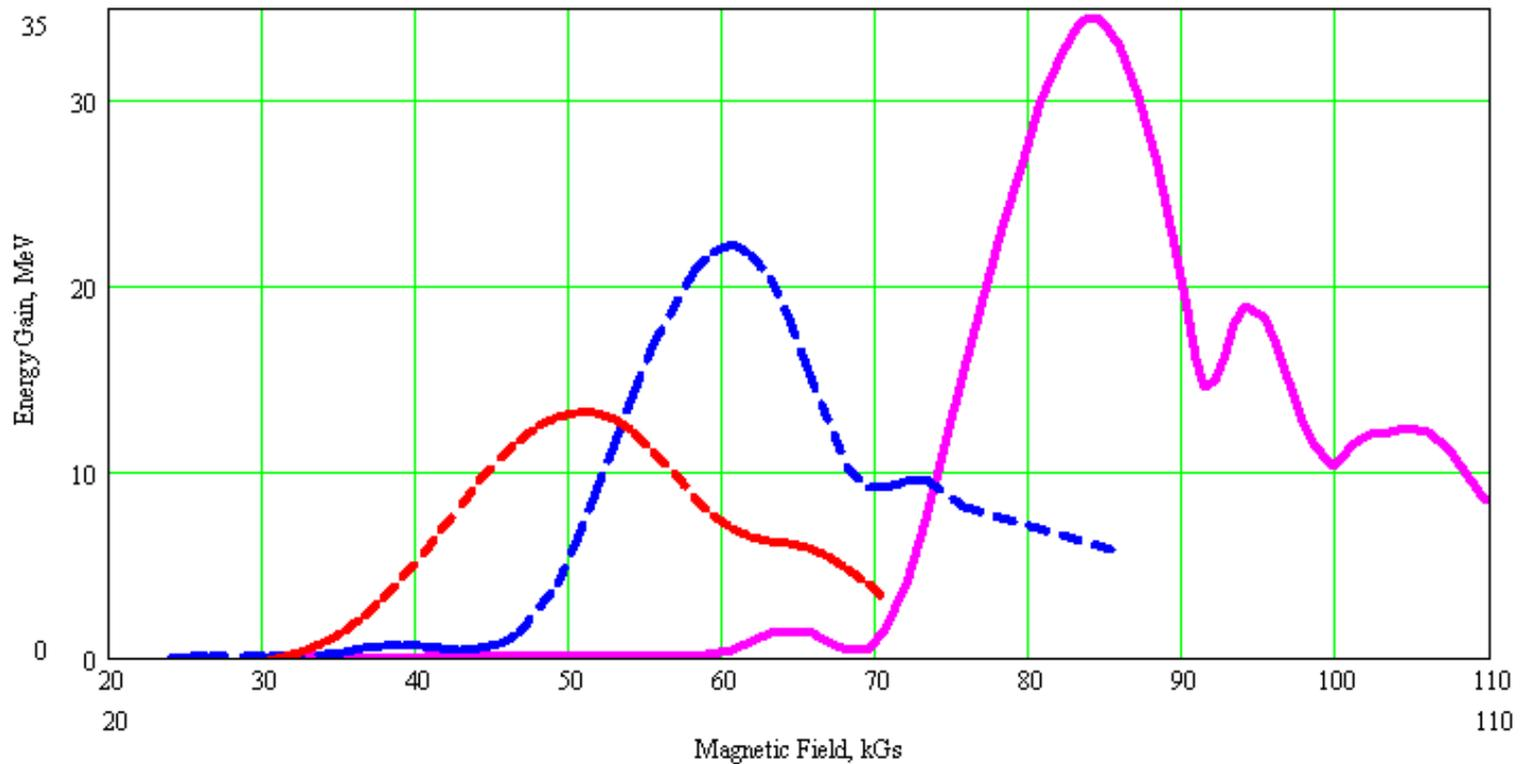
**FIG 1: Energy gain (MeV) vs. the maximum magnetic field (kGs) when the laser power is always 0.8 TW (the laser light is focused in the magnet middle plane with  $w = 1.3$  mm)**
