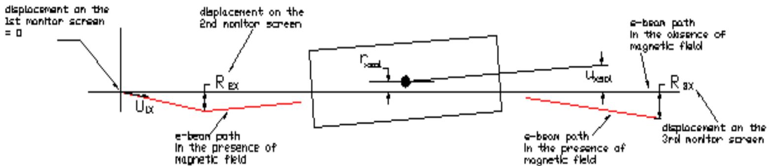
**Note: the e-beam path in the absence of the magnetic field coincides with the HeNe path, and is called the axis.**
