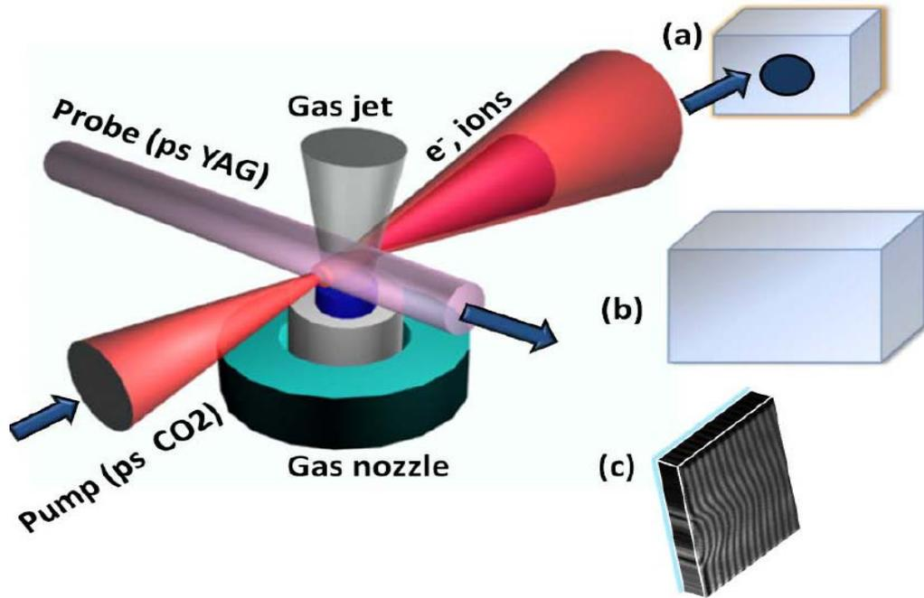
(a) Ion detection, (b) Magnetic field detection, (c) Diagnostics for interferometry
