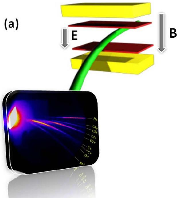
Typical ion traces from Al foil due to TNSA
