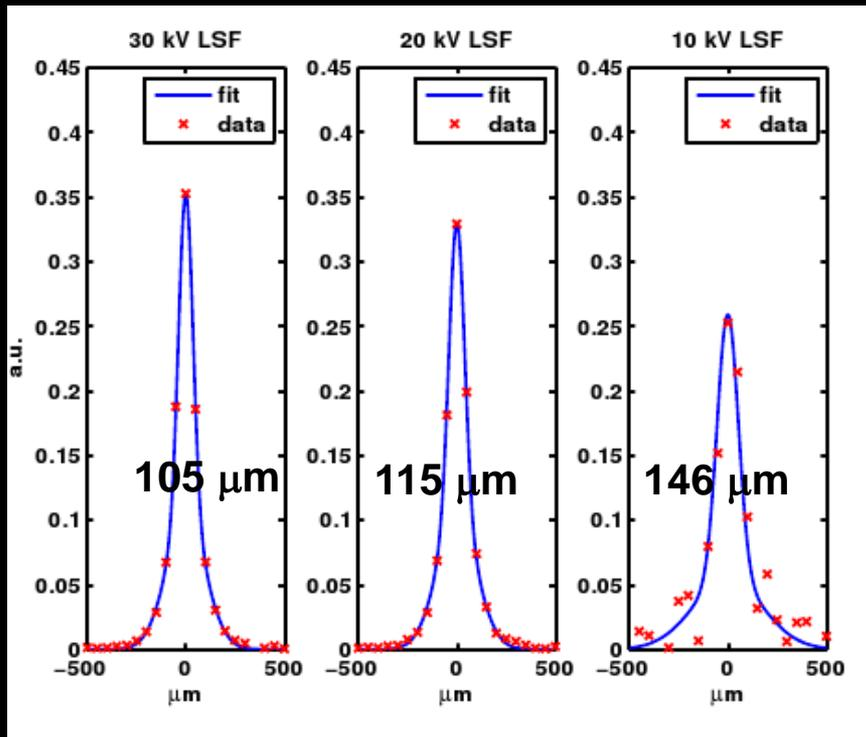
Resolution function measured by means of the Edge Response Function
