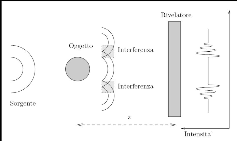
The shifted wave propagates in free space up to the detector.
