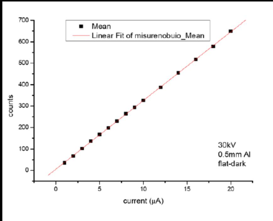
Linearity verified by means of an X-ray tube
