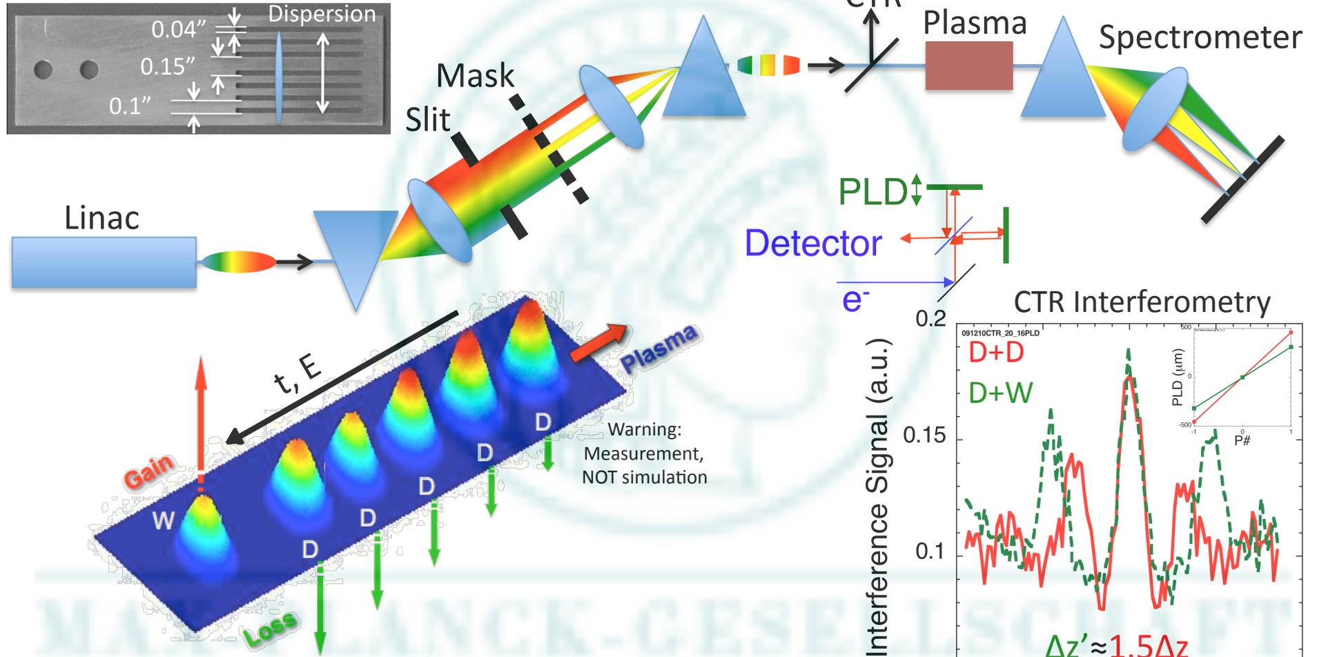
→ Choose beam parameters with mask and beam parameters:  $N$ ,  $\Delta z$ ,  $\sigma_z$ ,  $Q$
