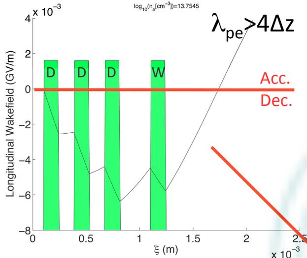
ulation (2D): microbunches with equal charge
