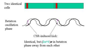
Figure 3: Transverse emittance cancellation mechanism - Half-integer phase advance.
