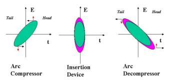
Figure 1: Longitudinal emittance cancellation mechanism.
