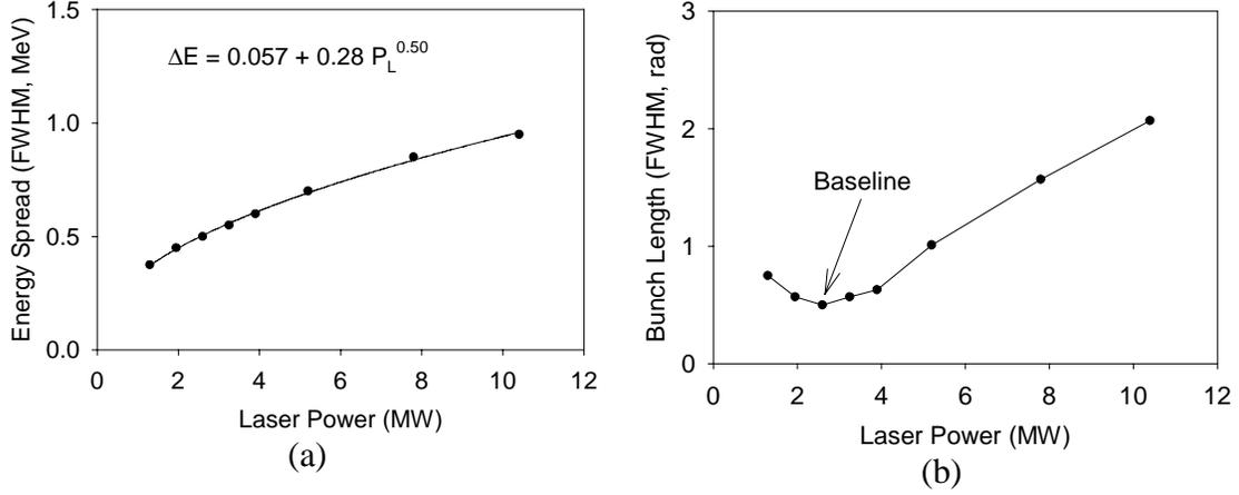
**FIGURE 5.** Scaling of induced energy spread and bunch length with laser power delivered to IFEL (a) Laser-induced energy versus laser power. (b) Bunch length versus laser power.
