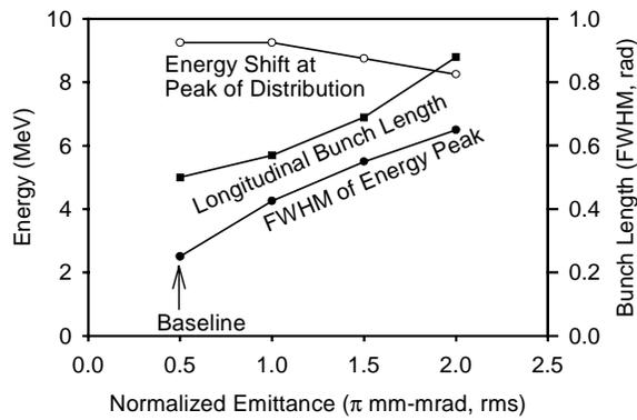
**FIGURE 7.** Scaling of ICA acceleration parameters with  $e$ -beam emittance.
