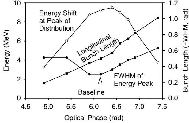
**FIGURE 9.** Variation of ICA acceleration parameters due to phase variation between electron microbunch and laser beam.
