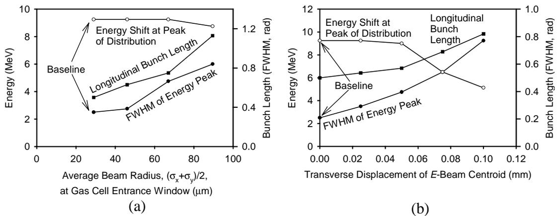
**FIGURE 8.** Scaling of ICA acceleration parameters with (a)  $e$ -beam size and (b) displacement.
