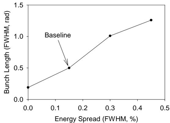
**FIGURE 4.** Scaling of bunch length with  $e$ -beam energy spread.
