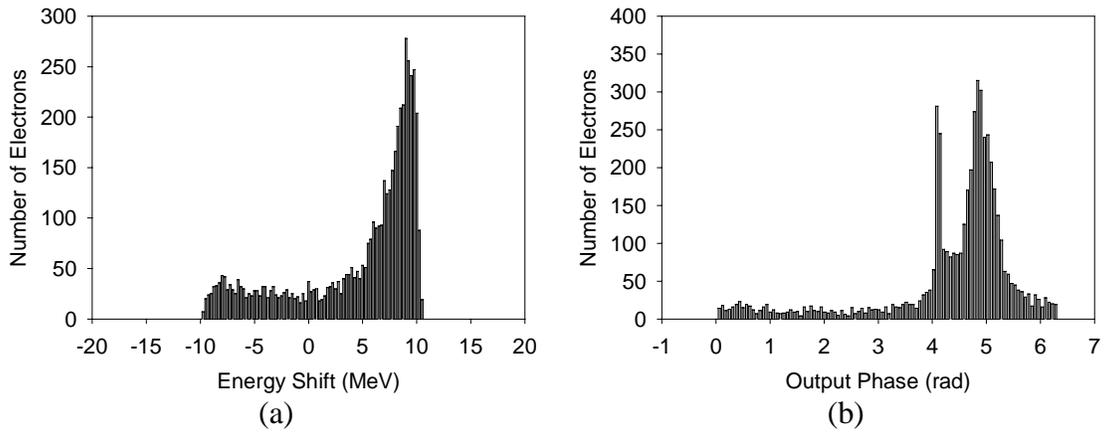
**FIGURE 6.** Output of ICA accelerator for  $E = 45$  MeV,  $\varepsilon_n = 0.5 \pi$  mm-mrad rms,  $\Delta E/E = 0.15\%$  FWHM, 1- $\mu\text{m}$  windows, with gas scattering. (a) Energy spectrum. (b) Longitudinal density.
