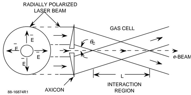
**FIGURE 3.** Basic geometry for inverse Cerenkov accelerator. From Ref. (6).
