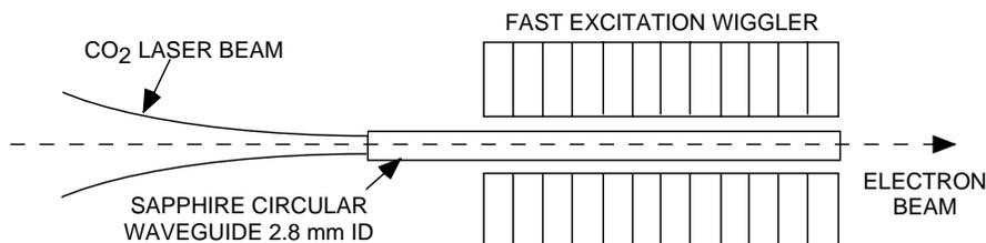
**FIGURE 2.** Schematic layout for BNL IFEL experiment.
