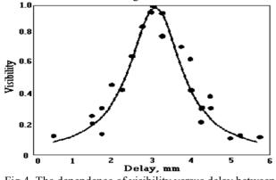
Fig.4. The dependence of visibility versus delay between two arms
