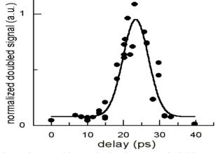
Fig.5. The second harmonic signal versus optical delay
