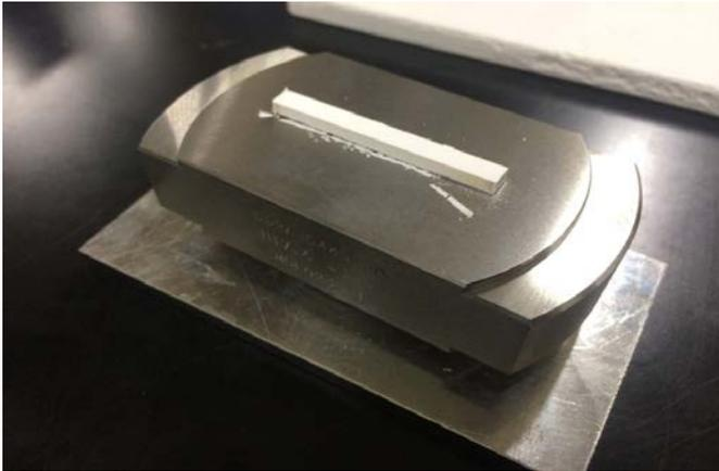
Part of sintering process at RIKEN to form solid  $\text{ZrO}_2$  targets for EBIS
