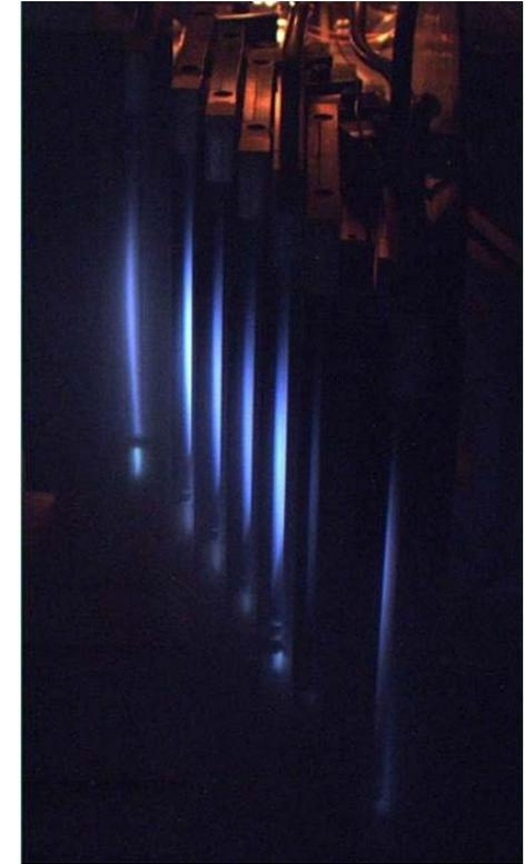
Electromagnetic separation of  $^{96}\text{Ru}$ . Image courtesy of ESIPP at ORNL.
