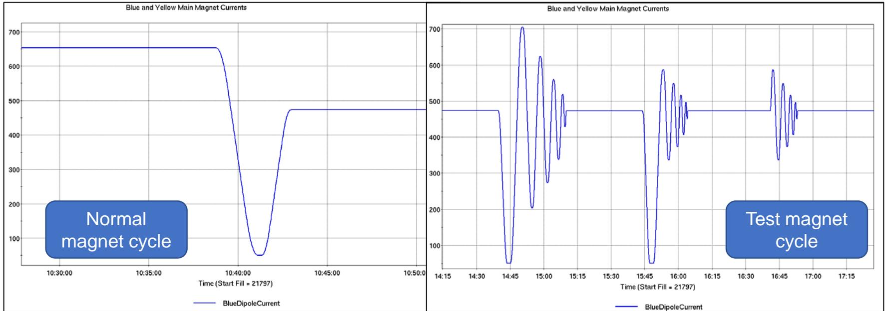
Hysteresis cycles: extra “wiggles” intended to reduce amplitude of persistent current drift, and minimize sextupole component in main dipole magnets
