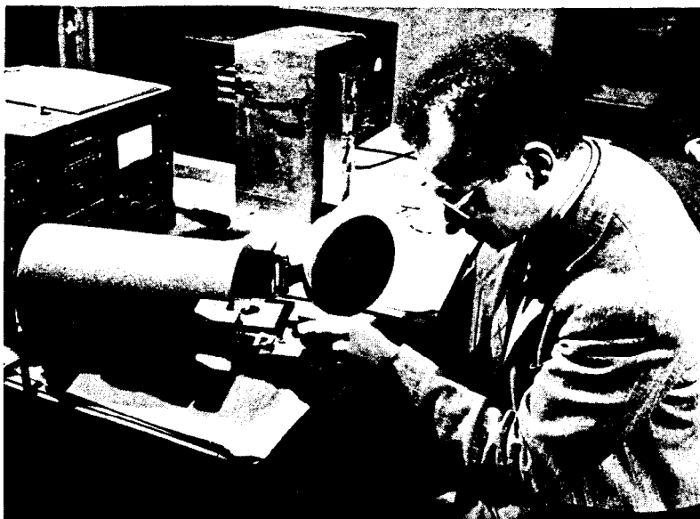
Dr. G. Friedlander placing a sample of radioactive nickel under a Geiger counter enclosed in a lead shield to measure its radioactivity. The box behind the lead shield contains the power supply and the scaling circuit for the Geiger counter.
