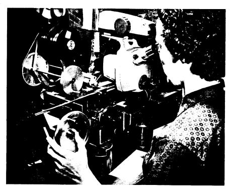
Some of the techniques for studying the properties of elementary particles depend upon observing and measuring photographs of tracks made by the particles in passing through matter. The people who make the observations and measurements are called "scanners". About a dozen scanners are employed at the Laboratory, and others are at work for experimenters from the Universities using the Cosmotron.
