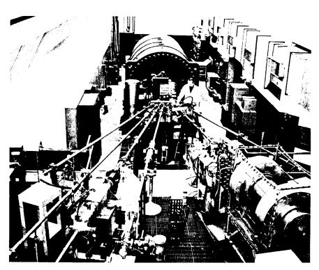
The Van de Graaff accelerator, located inside the pressure tank in the background, produces a charged-particle beam that may be bent into any one of the pipes and brought out to experimental set-ups in the foreground. Bob Lindgren is opening a valve near the beam-deflecting magnet and Arthur Timpe is making adjustments on a beam-pulsing oscillator in the foreground.
