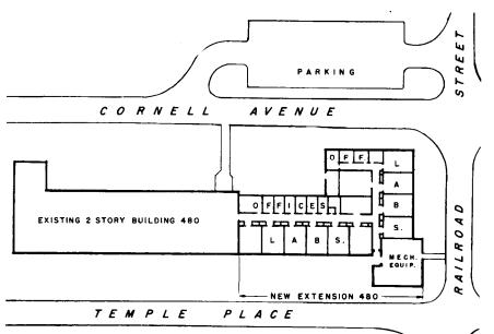
Excavation is well under way and the foundation has been started for an extension to the Metallurgy Building on Cornell Avenue. The extension will approximately double the work area of the existing building. It is expected that the extension will be completed by February, 1962 at a cost of approximately \$650,000. The construction contractor is the Anderson Construction Company. The architect-engineer is Walter Kidde Constructors, Inc.
