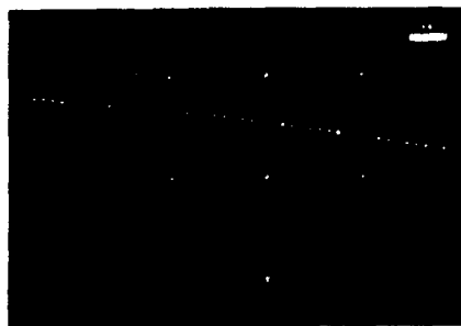
Photograph of a neutrino collision in the 10-ton aluminum spark chamber. The spark tracks show a long straight mu-meson created by an incident neutrino. Another track is also seen to point towards the origin of the event. This is thought to be a gamma-ray.
