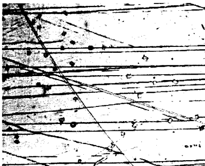
Polished surface showing Neumann lines, a twinning of the iron-nickel alloy produced by mechanical deformation, perhaps formed by the violent impact of an asteroidal collision.
