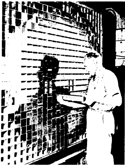
A technician at the Los Alamos Scientific Laboratory inserts core materials in one of the two matrices of the "Honeycomb" critical assembly machine. The core materials are part of a nuclear propulsion reactor mockup. The two halves are remotely brought together and the nuclear properties of the core can be measured.
