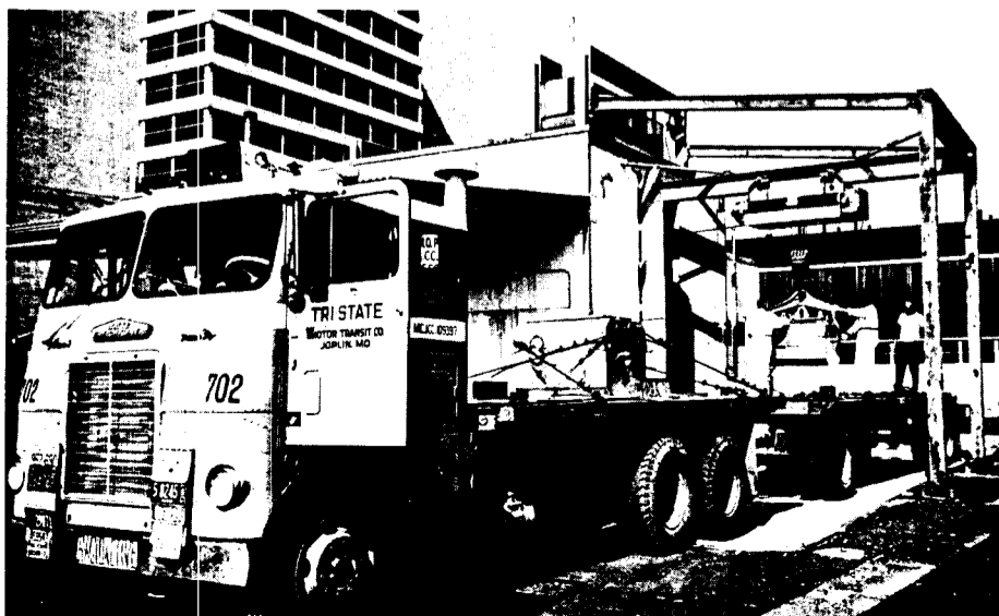
Loaded casks are placed on a special truck for shipment to the AEC's Savannah River Plant where uranium metal will be recovered and fission products will be removed.
