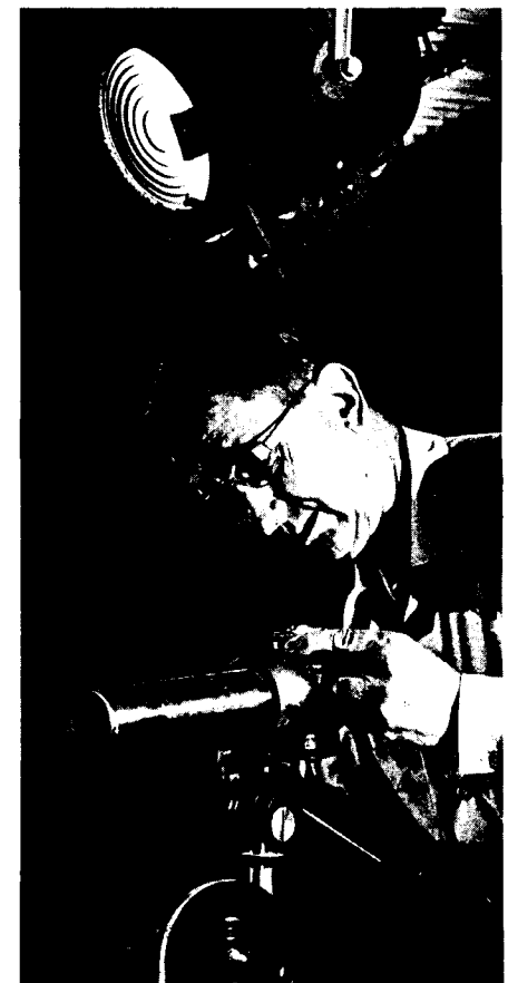
Bud Pollock takes no chances when it comes to radiation. When he calibrates an instrument he reads the scale from a distance through a small telescope.
