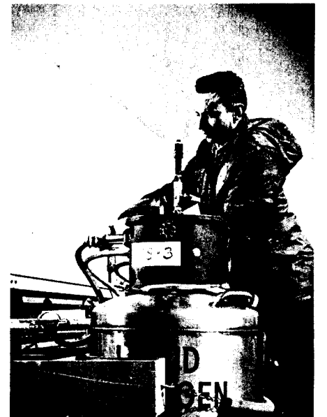
Charles Frank, fills a 175-liter vacuum insulated tank from the BNL 40,000-gallon liquid hydrogen storage facility.
