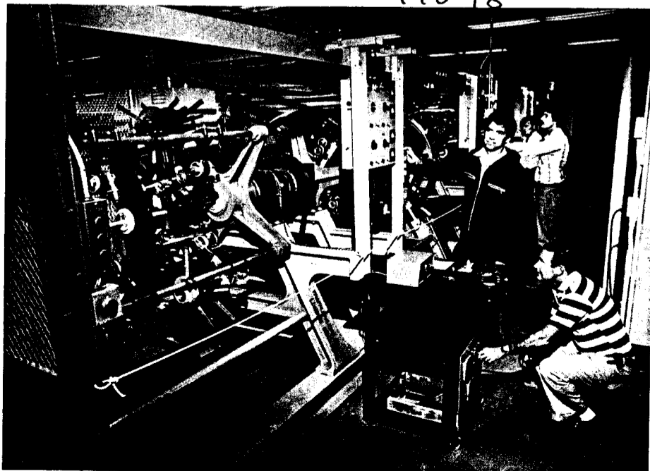
In the winding room, Tom Muller (center) operates the winding machine, while Bob Kowalski (right) applies tension control to the taping heads. At rear, Hank Noehren (left) and Kevin Stevenson observe other sections for proper operation. —photos by Reben
