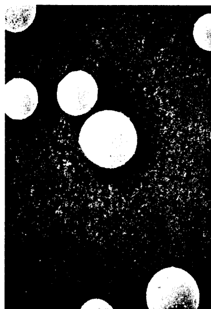
Rare-earth oxide spheres 100 microns in diameter reveal a wealth of microstructural detail to Instrumentation's new scanning electron microscope. The right-hand image shows an enlarged view of the central sphere at 20,000X with a resolution of 50 angstroms.
