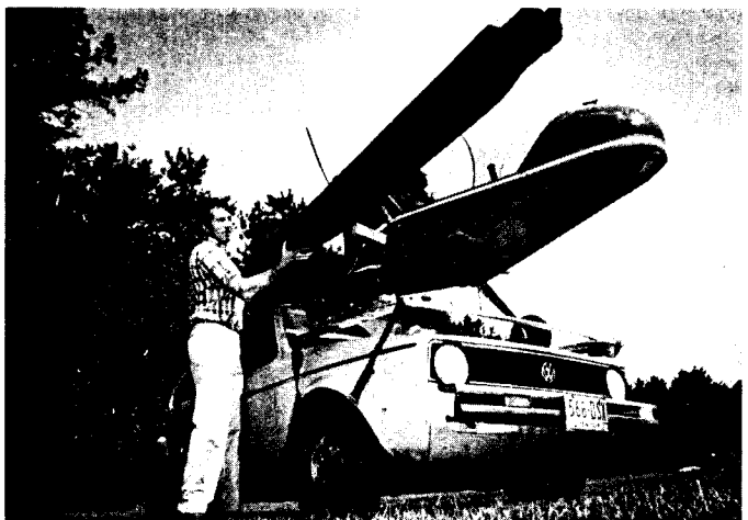
Rodger transports his ultralight on top of his compact car. It breaks down into three basic units — two 19-foot wings, which disassemble and fold into bags, and the fuselage, or main body of the plane. Starting with the pieces all on the ground, assembly time is only eight minutes.
