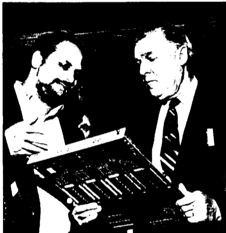
Central to experiment 787's electronics is the transient digitizer board that Physicist Maged Atiya shows to Secretary Watkins. Using commercial analog-to-digital chips, this 500-megahertz, Fastbus transient digitizer was designed and produced by BNL.
