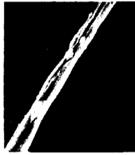
Above: "Necking and sausaging" in niobium-titanium filaments.
