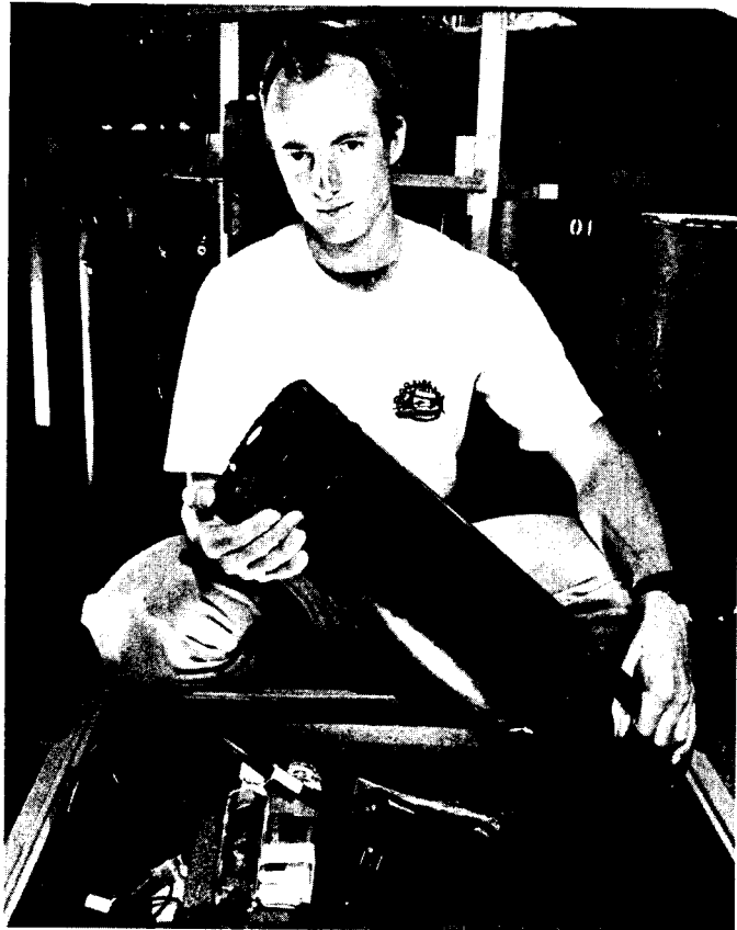
Mike Behrenfeld, Department of Applied Science, holds a fast repetition rate fluorometer of the type that he used on a recent cruise near the Galapagos Islands to measure phytoplankton activity before and after iron was added to the water.
