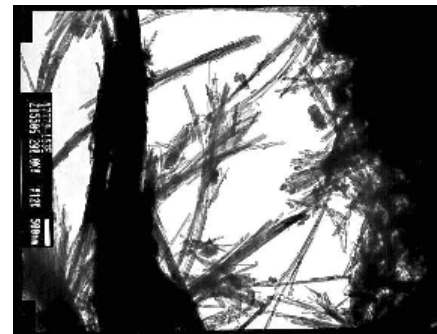
At left, a magnified image of asbestos-containing fireproofing taken through a BNL electron microscope. At right, the same material after treatment with the BNL-Grace process — the asbestos fibers have been chemically changed into amorphous minerals.
