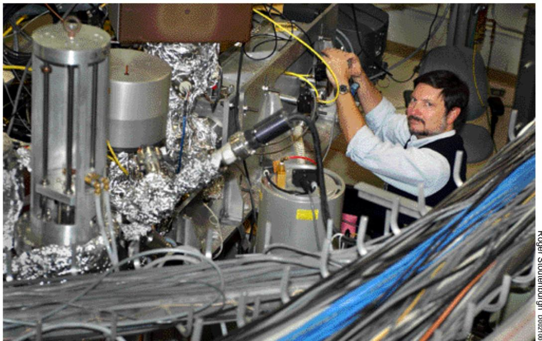
Larry Carr, National Synchrotron Light Source (NSLS) Department, is in front of the far-infrared spectrometer at beamline U12IR of the NSLS's Vacuum Ultraviolet ring.
