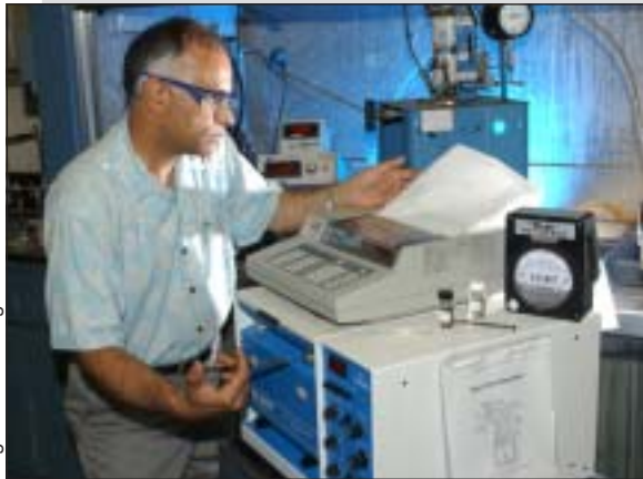
Devinder Mahajan uses a gas chromatograph to analyze carbon monoxide levels in hydrogen purified using his patented process.
