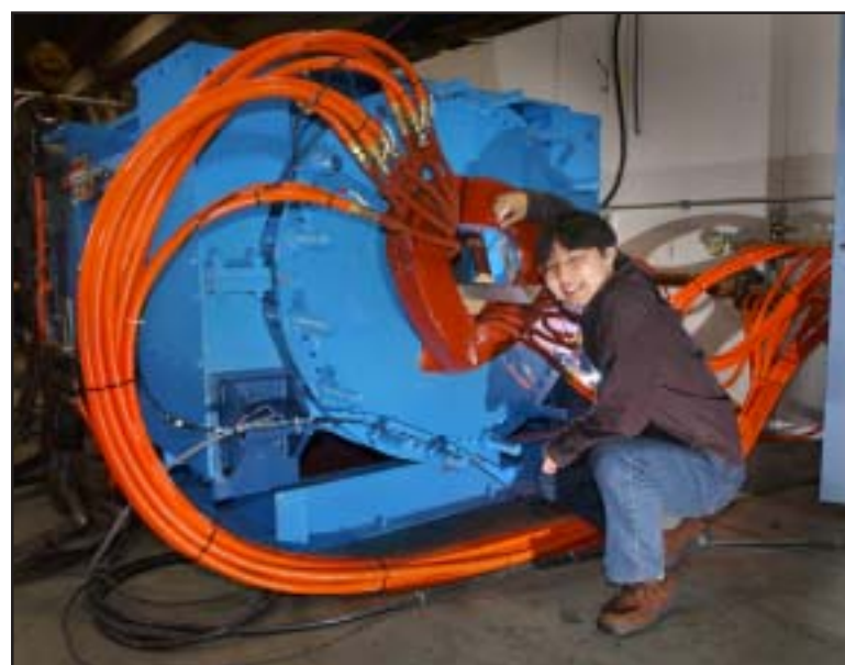
Pictured with the new warm helical Siberian snake magnet is Junpai Takano of the Tokyo Institute of Technology, who designed the magnet with Masahiro Okamura of RIKEN. Built by the Takano Original Magnet Company in Japan, the new snake was funded by RIKEN.
