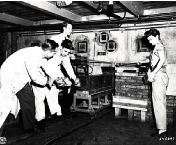
March 1948: “Dr. Ralph Overman removes a bombarded sample from a carrier block from the Brookhaven Graphite Research Reactor. Mrs. Weber measures the samples’ radioactive strength.”
