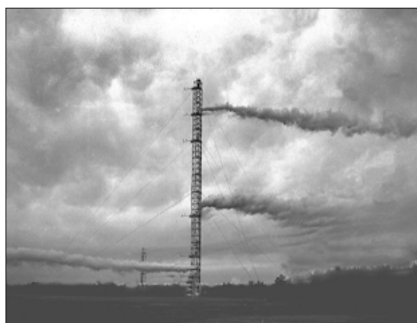
A 1951 smoke run of three smoke devices from ground and tower. Note the change in wind direction at different levels.
