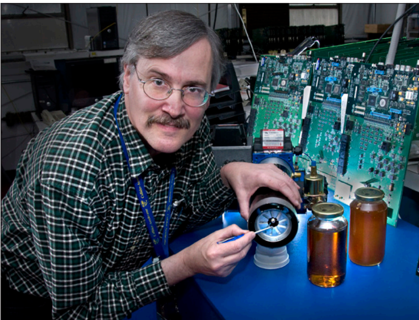
Ron Schroeder points to the main component of his home-heating recycled cooking-oil burner.
