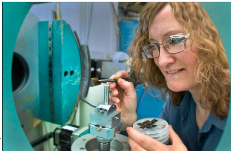
IBM's Jean Jordan-Sweet loads a silicon wafer sample into the diffractometer at NSLS X20A for colleagues performing a remote access experiment.
