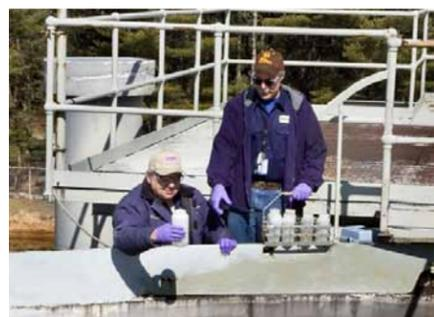
**STEP 3.** Aeration reduces carbon dioxide gas and aids in iron oxidation. At the aeration tank, Phil Pizzo and Greg Stawski are seen sampling the water.
