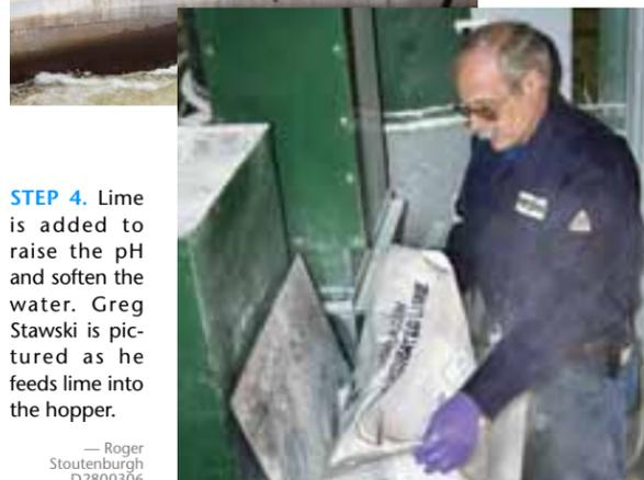
**STEP 4.** Lime is added to raise the pH and soften the water. Greg Stawski is pictured as he feeds lime into the hopper.
