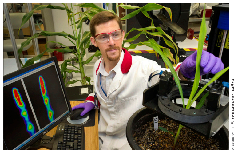
Goldhaber Fellow Ben Babst with a prototype of a positron emission tomography (PET) device for imaging plants. This device is being designed and built through collaboration between BNL's Medical and Physics Departments, its Instrumentation Division, and Sherbrooke University in Canada.
