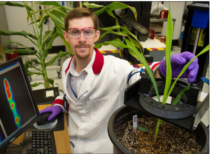
Above: Ben Babst with a prototype of a positron emission tomography (PET) device for imaging plants. This device is being designed and built through collaboration between BNL’s Biosciences and Physics Departments, its Instrumentation Division, and Sherbrooke University in Canada.
