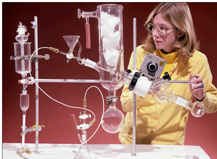
BNL chemist Joanna Fowler with an early 18 F-DG synthesis apparatus
