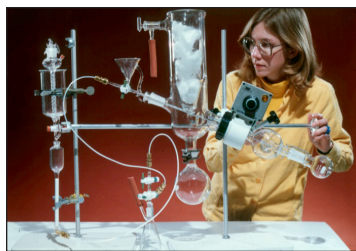
Early ^{18}\text{F} FDG synthesis apparatus
