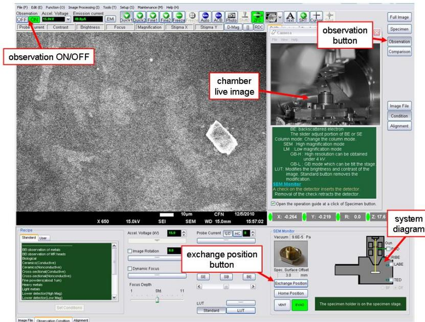
FIG. 3. Main window of Graphical User Interface (GUI).
