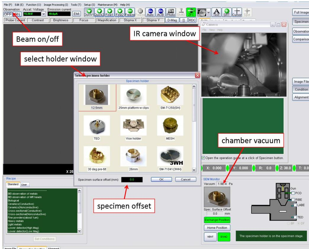
FIG. 9. Graphic user interface showing the specimen holder popup window.
