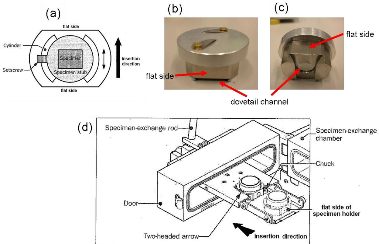
FIG. 4. Locking the sample holder in place in the airlock chamber. a) Top view of specimen holder. b) and c) Identification of "flat side" with respect to dovetail channel at the base of holder. The flat side is perpendicular to the length of the dovetail channel. d) Correct way of locking specimen holder with the holder's flat side perpendicular to the insertion direction. (Diagrams taken from JEOL's manual.)
