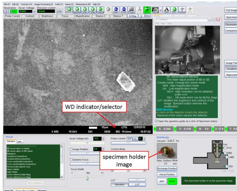
FIG. 10. Graphic user interface showing the position of the WD indicator/selector area.
