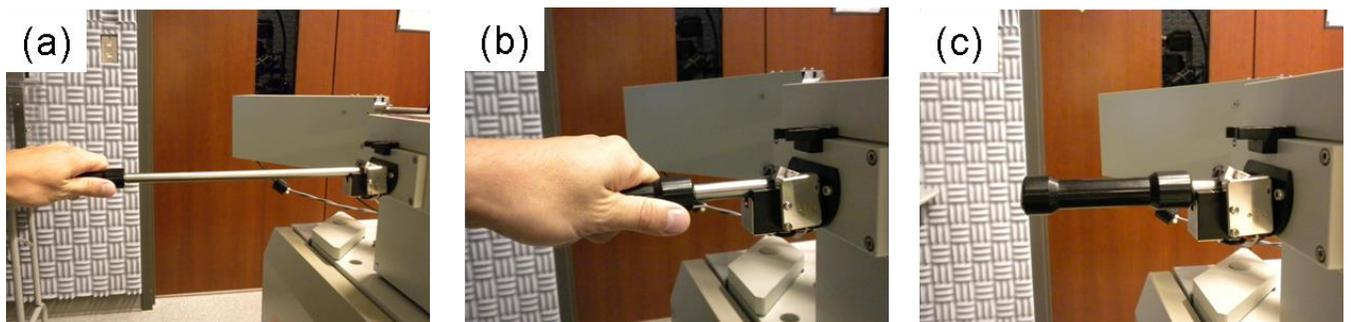
FIG. 7. Locking holder in SEM stage. (a) Insertion of rod by pushing horizontally along rod's axis. (b) Rod position when it first touches the SEM stage. (c) Rod position with holder locked in SEM stage.
