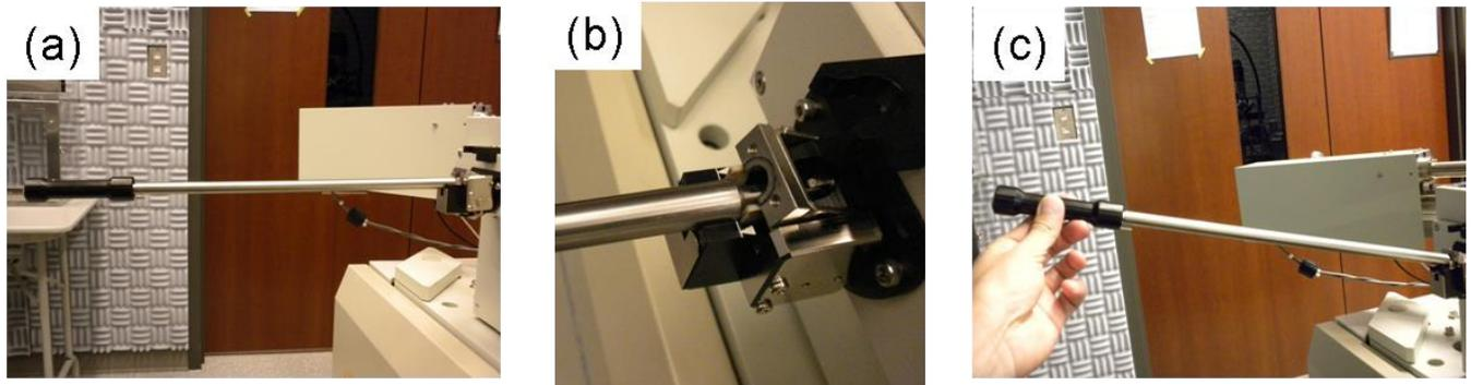
FIG. 8. Retracting exchange rod. (a) Fully retracted and resting on the plastic stopper. (b) Detail of rod resting on plastic stopper. (c) Lifting of rod to its vertical position without using any force along rod's axis.
