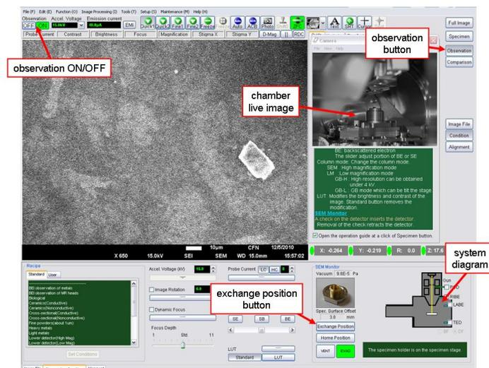
FIG. 12. Main window of Graphical User Interface (GUI).
