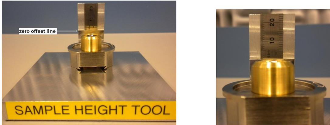
FIG. 2. Sample height tool. The right image shows a sample correctly flushed at the zero offset line.
