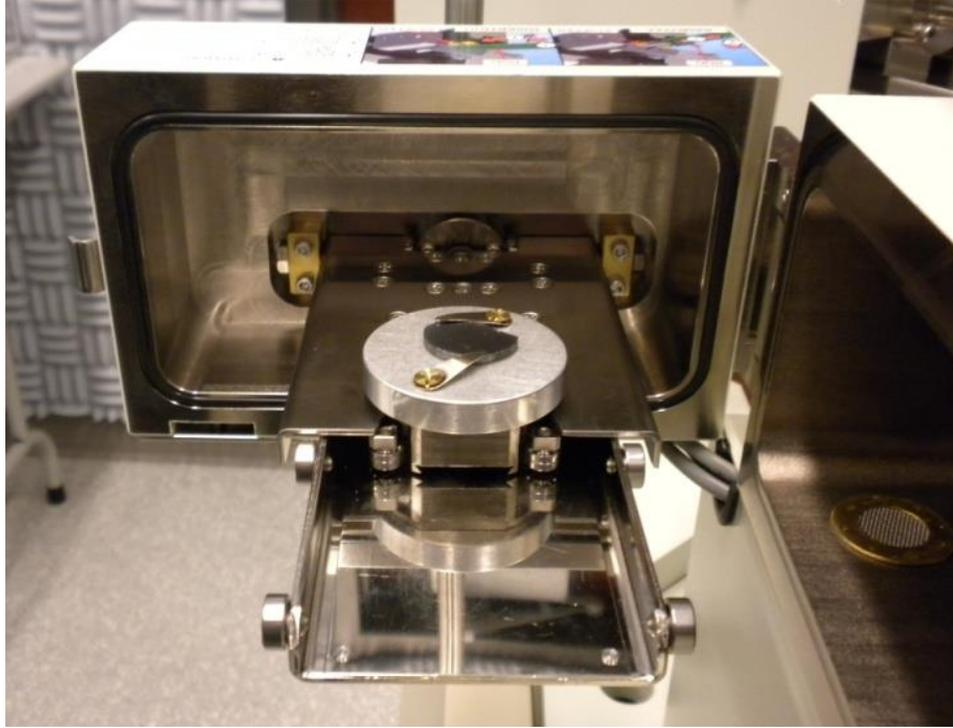
FIG. 5. Sample locked in place in the airlock chamber
