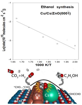
**Top:** Arrhenius plot for ethanol synthesis from  $CO_2$  and  $H_2$  at 0.5 atm of  $CO_2$  and 4.5 atm of  $H_2$ ; **Bottom:** Structures of Cu-Cs-ZnO interface on Cu/Cs/ZnO(0001) surface, active for C-C coupling and ethanol synthesis.
