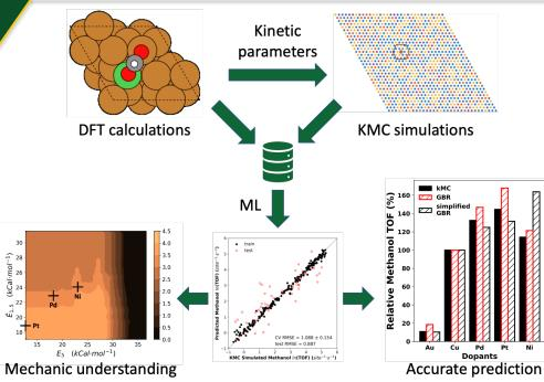
Schematic for the proposed data-driven framework, a case study of identifying and interpreting activity-controlling descriptors in CO hydrogenation to methanol over Cu-based alloys.
