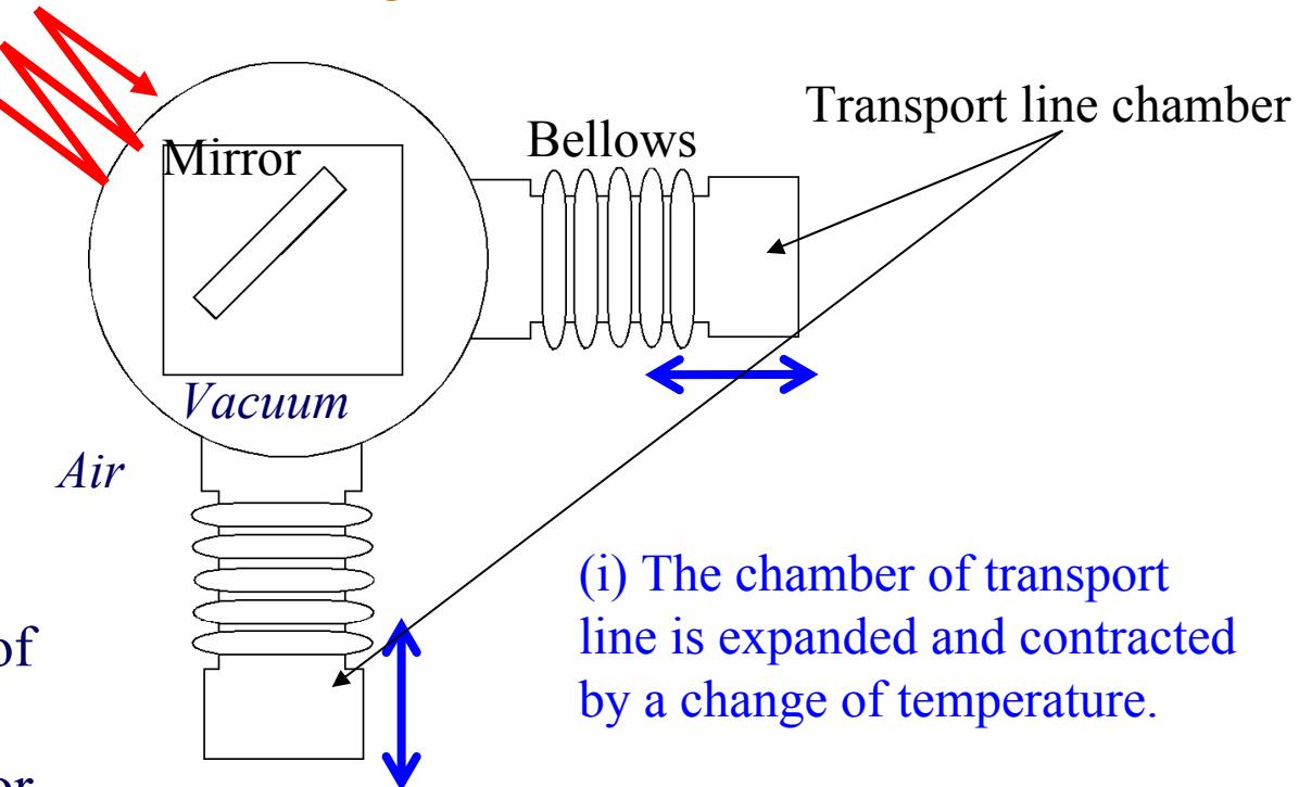
• In the chambers... Vacuum → Atmospheric pressure N<sub>2</sub> gas.
