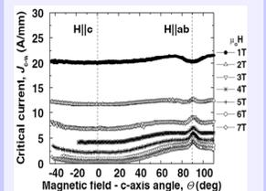
Strong and isotropic flux pinning in the 3- $\mu\text{m}$ -thick record high  $J_c(H)$  and  $T_c$   $\text{YBa}_2\text{Cu}_3\text{O}_7$  (YBCO) films at liquid  $\text{N}_2$  temperature. - Soloviyov, et al
