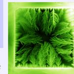
Magneto-optical image of flux in C-doped  $\text{MgB}_2$  superconductor - Li et al
