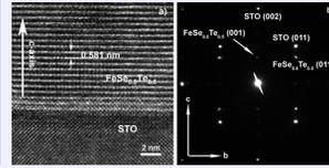
High resolution TEM & elec. diff. pattern of superconducting  $\text{FeSe}_{0.5}\text{Te}_{0.5}$  thin film.
