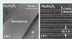
High resolution TEM images of oxide thermoelectric films on Si and glass (not shown). This work opens the potential of
