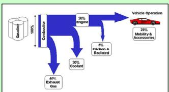
Fig. 1 Typical energy path in gasoline fueled internal combustion engine vehicle (Source: GM)
