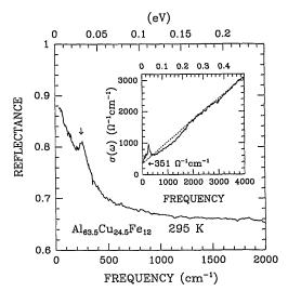
Fig. 7. Reflectance of Al<sub>63.5</sub>Cu<sub>24.5</sub>Fe<sub>12</sub> at 295 K from 30 to 2000 cm<sup>-1</sup>. The inset shows the Kramers–Kronig optical conductivity over the same frequency range. The dashed line in the inset is the extrapolation of the conductivity to zero frequency. The value of the intercept is close to the measured dc conductivity for this material.
