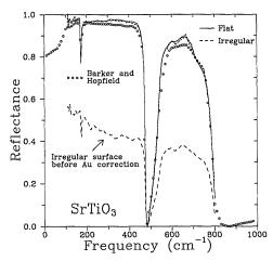
Fig. 6. Reflectance of SrTiO<sub>3</sub> measured on the irregular sample shown in Fig. 5, short-dashed curves; a large polished sample of the same material, solid curve; data from Barker and Hopfield,<sup>7</sup> circles. The curve with the long dashes shows the signal from the irregular sample referenced to a flat mirror.
