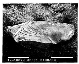
Fig. 5. Irregular piece broken from a crystal of  $SrTiO_3$  used to measure the spectra in Fig. 6.
