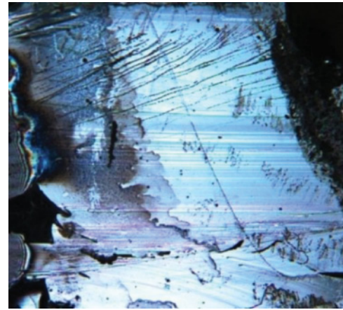
FIG. 3. (Color online) A photomicrograph of the cleaved ab -plane surface of \text{La}_{1.875}\text{Ba}_{0.125}\text{CuO}_4 revealing a number of striations and cleavage steps; the total area shown is roughly 2 \text{ mm} \times 2 \text{ mm} .
