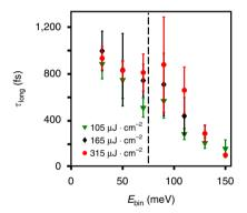
Figure 7 | Experimental fluence and energy dependence of  $\tau_{long}$ .  $\tau_{long}$  versus  $E_{bin}$ , as defined in the main text, for  $\Phi = 105$  (green) 165 (black) and 315 (red)  $\mu$ J·cm $^{-2}$ . The vertical dashed line at 75 meV denotes the theoretical position of  $+\hbar\Omega$ .
