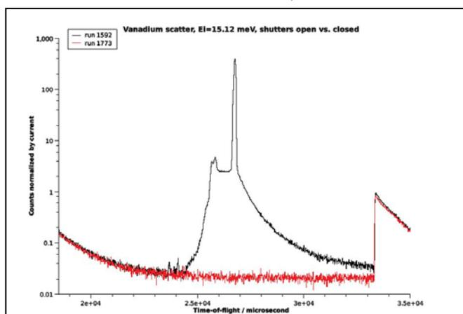
**Figure 1.** Intensity from Vanadium rod sample integrated over the HYSPEC detector array with open (black) and closed (red) primary and secondary shutters.
