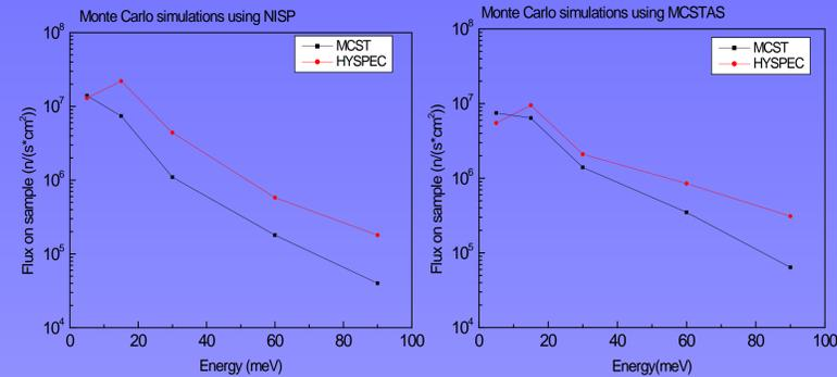
Comparison of the neutron current through 2 cm tall sample provided by the hybrid model (red) and a traditional time-of-flight scheme (black)
