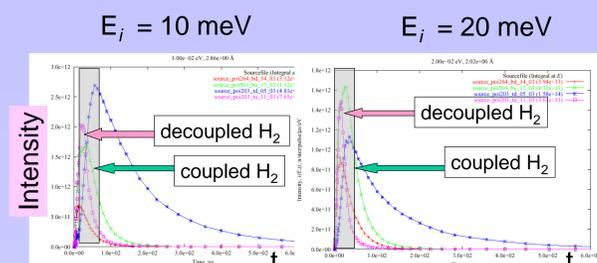
Coupled supercritical hydrogen. Figure of merit is the integral flux within 30-50  $\mu$ s time window, defined by the length of the secondary flight-path
