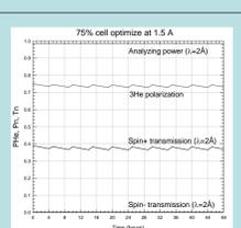
Optical pumping may be difficult due to the shape of the cell. Refilling may be the solution. Filling station example: Max <sup>3</sup>He polar. = 0.75, optimized at 1.5 Å. T1 = 200 hours, refill 75% volume every 5 hours. (Plot: for 2 Å neutrons)
