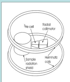
2 pairs of coils with diameter 400 mm & 350 mm separated by 400 mm. By applying appropriate currents to the coils, field uniformity similar to a pair of 400 mm diameter Helmholtz coils can be obtained.
