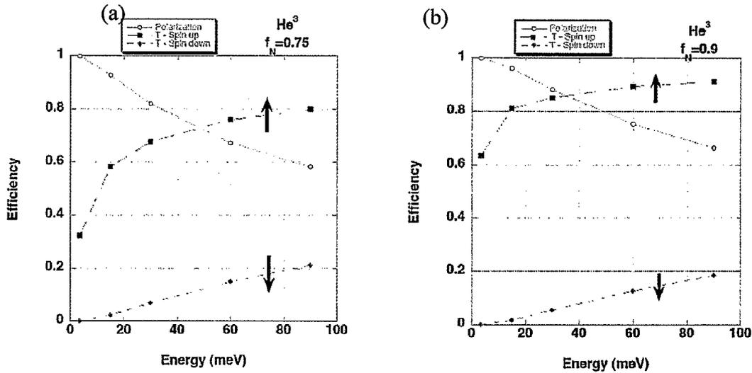
Figure 5: Calculated polarization and transmission for  $\text{He}^3$  spin filters with nuclear polarization (a)  $f_N = 75\%$  and (b)  $f_N = 90\%$ .
