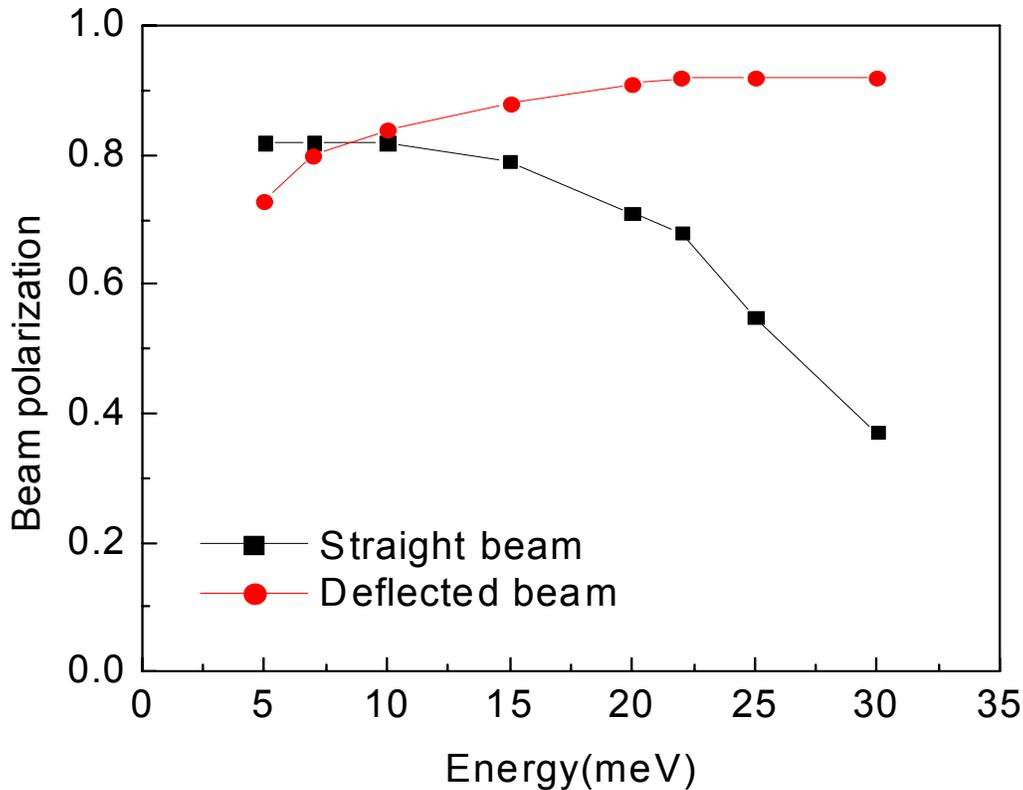
Figure 4. Average beam polarization in each of the two beams
