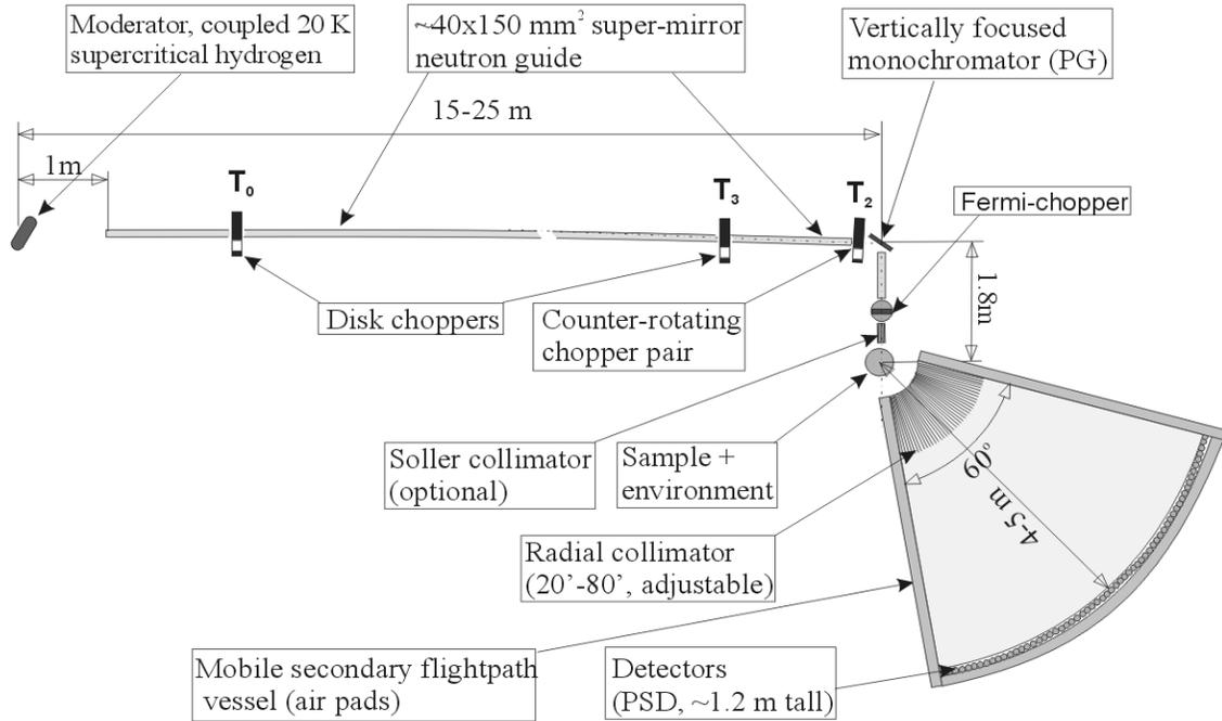
Figure 1 Schematic showing HYSPEC's principle elements.
