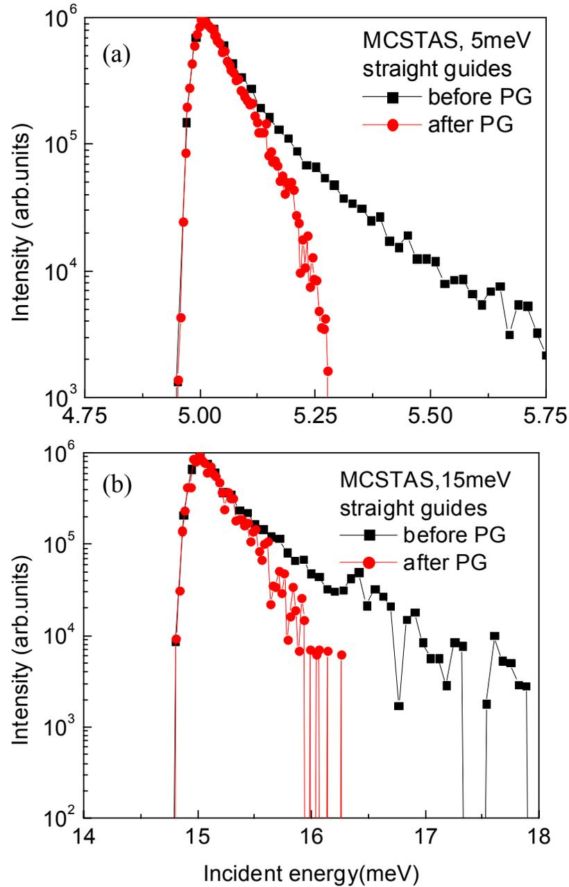
Figure 2. Incident neutron spectrum before and after reflection from a PG monochromator; (a)  $E_i = 5$  meV; (b)  $E_i = 15$  meV.
