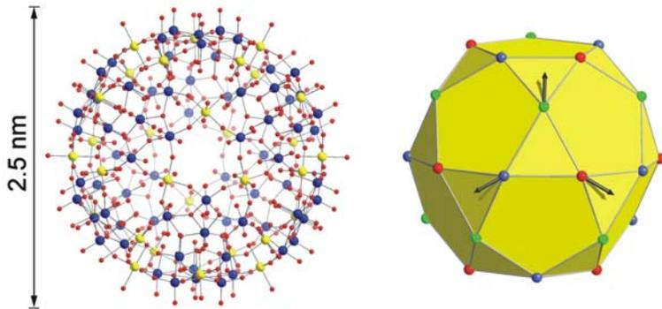
Figure 2.4. Structure of the  $\{Mo_{72}Fe_{30}\}$  molecule (left; Mo: blue, Fe: yellow, O: red) and the inscribed  $Fe_{30}$  icosidodecahedron (right; the classical ground state is characterized by three spin vector subsets [blue, green, and red Fe centers]). In certain targeted derivatives, all or a part of the thirty Fe(III) centers will be replaced by different di- and tri-valent paramagnetic ions.
