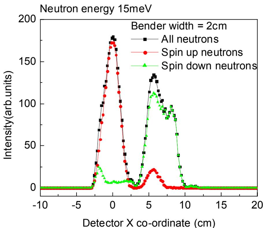
Figure 3. Spatial distribution of two neutron polarizations on the detector as created by a single supermirror-bender
